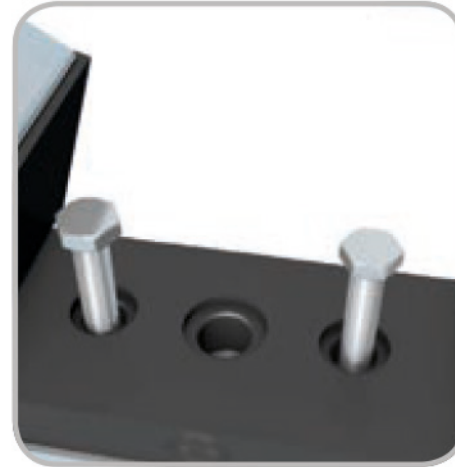
3 Secure cleat to mounting surface using 2 x M10 or 1 x M12
